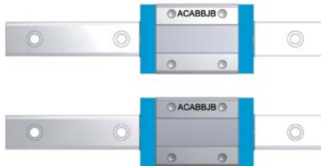
Figure 3.4 Marking the main and auxiliary guide
